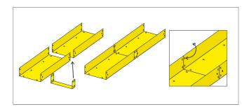
Joining two ducts together using the fasteners.
