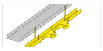
Example of fixing the ducts to existing structures.
