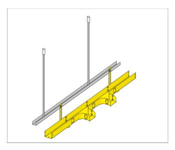
Installation to a ceiling (using additional bearing C-profile and anchor bolts.)
