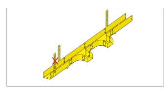
"L" shaped bearing elements should be placed only on one side of the duct thus allowing for easy loading of the fibre optic cable.
