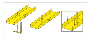
Joining ducts with bearing element, using carriage bolts.
